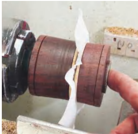
STEP 29. With the base mounted in the chuck now is the time to jam the lid on. If you find it's a bit loose you can use a piece of thin paper; this will ensure that the lid can't spin
